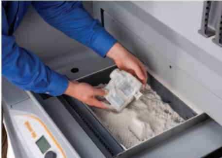
ZCorp's 3D printing technique uses a four-colour CMYK powder printing and binding process
